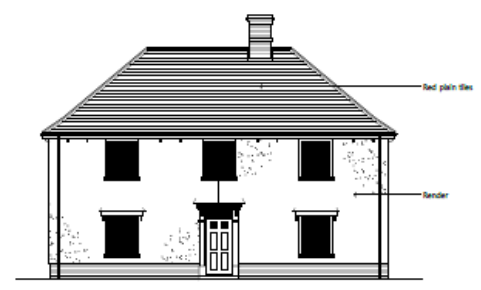
Front (north) elevation 1:100
