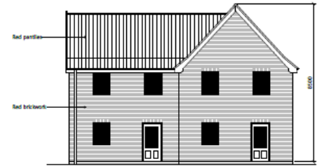
Rear (north) elevation 1:100
