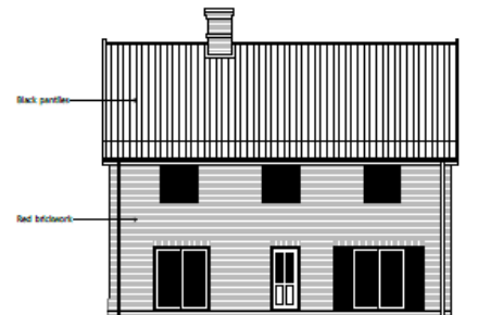
Rear (south-west) elevation 1:100
