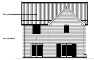
Rear (south-east) elevation 1:100
